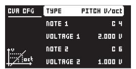
4. Set the **SRC** parameter of the CV A page to TR1. This will make the CV track send out pitch voltages according to the note trigs on synth track 1.
