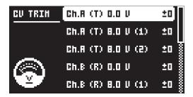
Each CV output has three trim settings. Begin by selecting 0 V, then press and hold the [YES] key. 0 V is output as long as [YES] is held down. Use [ARROW] keys [LEFT]/[RIGHT] or *DATA ENTRY KNOB A* to adjust the voltage until your voltmeter shows exactly 0 V. Repeat the process for both 8 V settings (the first one is for continuous voltage, the second is for pulse).
