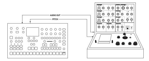
The CV/Gate outputs and the external inputs allow an external oscillator to be used with the internal Analog Four MKII oscillators. Use this trick when you want a different (perhaps old, quirky and unpredictable yet charming) oscillator to provide the fundamental tone but still want the control and modulation power of the Analog Four MKII.
