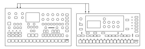
Thanks to the neighbor routing, all the filters of the Analog Four MKII can be used for providing an immense mono filter bank consisting of 8 filters plus 4 overdrive circuits. The setup can be either serial or parallel. It can, of course, be set up for stereo filtering as well. In this scenario, 4 filters are available for the left and right channels.
