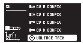
Make sure you have a good voltmeter before proceeding. Connect a TRS cable to the output you want to trim. Connect the voltmeter's negative terminal to the sleeve of the connector. Connect the positive terminal to the tip of the connector.
