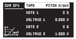
Please read the following paragraphs on how to set up CV pitch control. CV pitch is configured by finding the voltages generating two different notes from the synthesizer you wish to control. To get a good result, you should select the notes two or three octaves apart.
